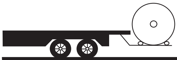
Reels should be lowered using hydraulic gate, hoise or forklift. LOWER CAREFULLY.
